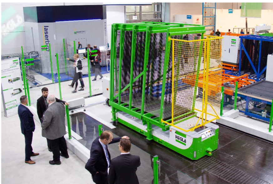
Image 4: With the Automated Guided Vehicle (AGV), glass transport is automated between individual stations and flexibly customised at any time - all part of cutting-edge shop floor logistics.
