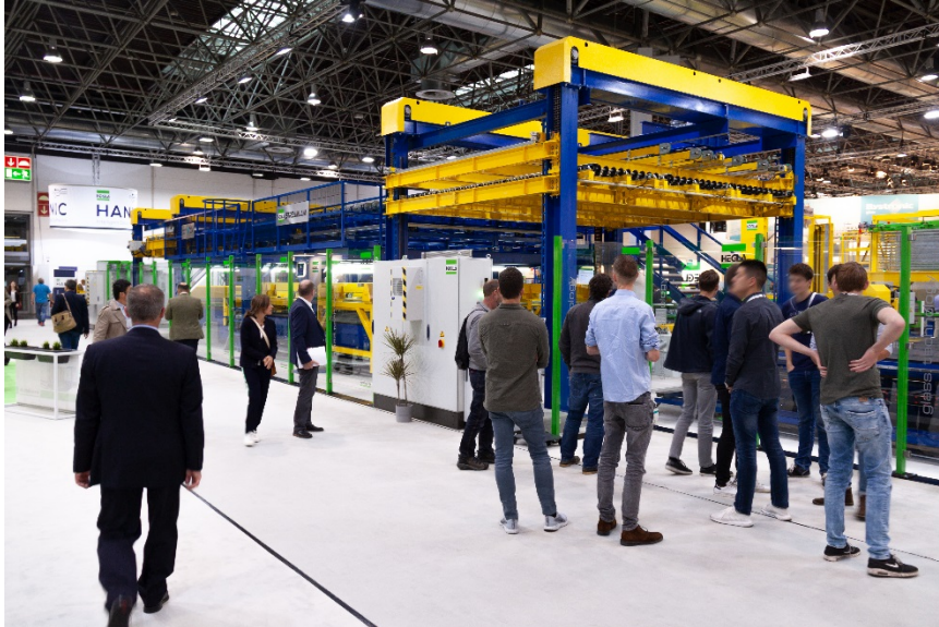
Image 1: With the promise of up to 30 percent more output compared to a conventional cutting line, the new high-performance cutting system for laminated safety glass, StreamLam, attracted a great deal of interest from visitors.
