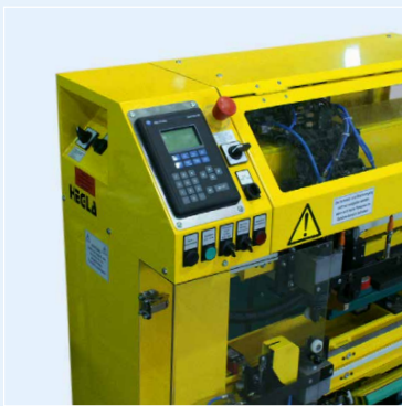
Display of the machine-status via "Panel View"
