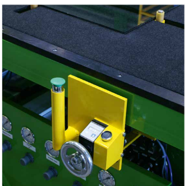
Manually moveable measuring stops with vernier adjustment
