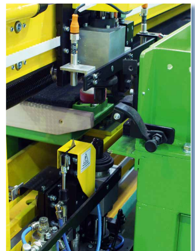
Precise double cutting head system for parallel top and bottom cut with knife separation for fast and clean PVB separation
